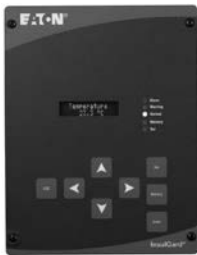
InsulGard Relay (PD Monitoring)
