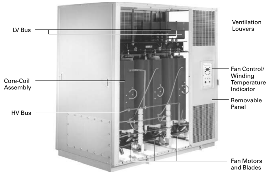
Cast Coil Substation Transformer
