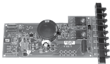
Contactor Control Board
