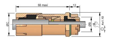
Our range of MARINE BVLE FS cable glands is a specific marine and Navy cable management solution as per DTCN 5975 CA standards.
