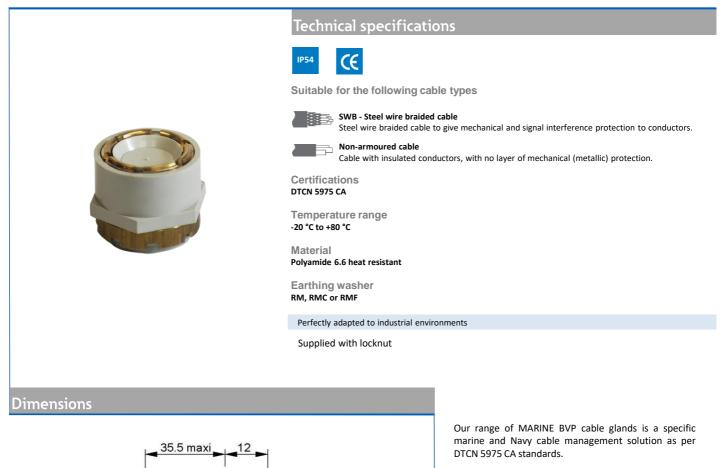
These low-tight cable glands allow the connection of non-armoured, and steel wire braided armoured cables.
