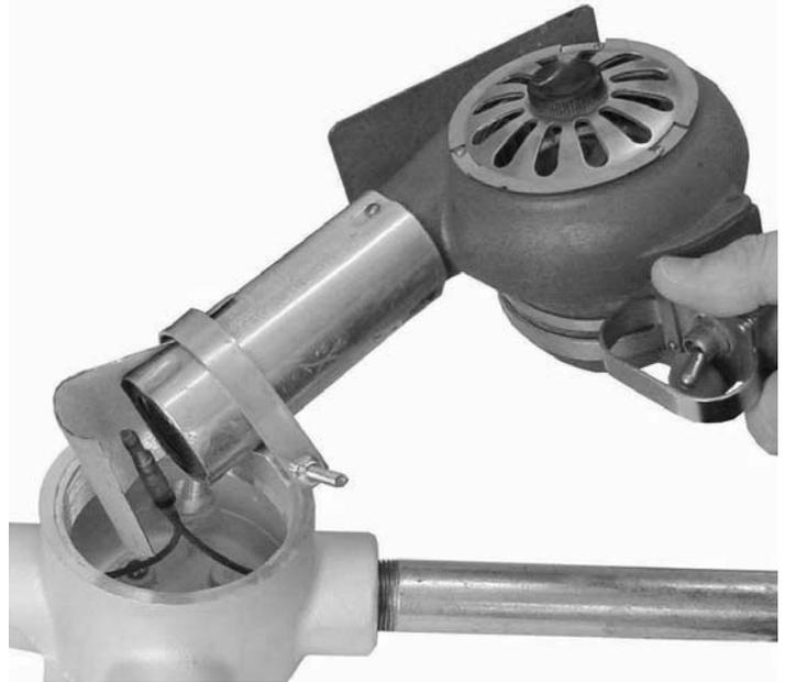
solder preform melts and flows into the turns of the conical copper coil. After the solder ring has completely disappeared, continue heating for 6 seconds.
