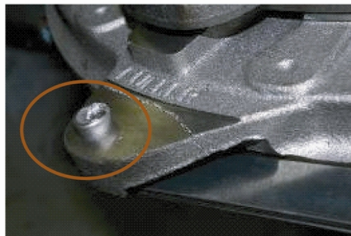
Damage to rivet from jackscrew
