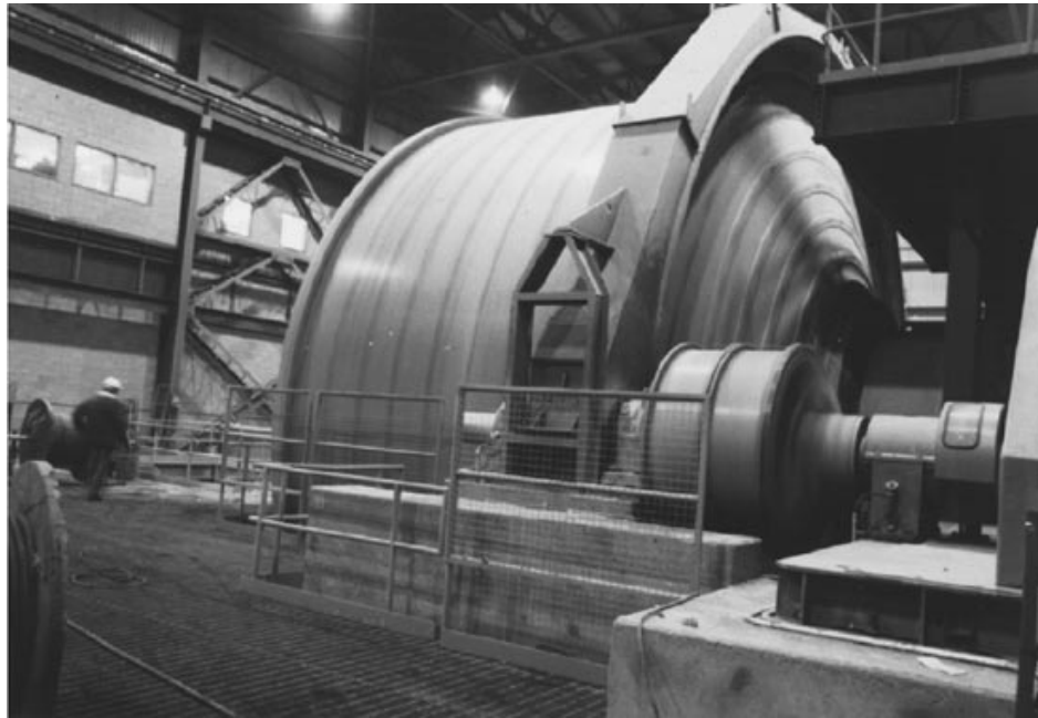
Dual VC clutch application on autogenous mill drive.
