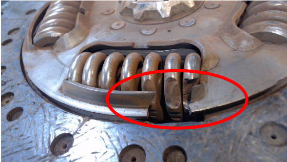
Broken spring cover
