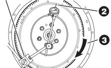
2 Put gage finger in contact with flywheel face near the outer edge.
