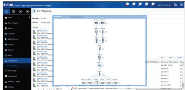
Port mapping allows users to view power, network and fiber connection throughout the data center to quickly perform failure and impact analysis
