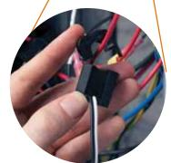
Clamp-on voltage sensors attach to existing branch circuits and monitor voltage while powering the electronics module.
