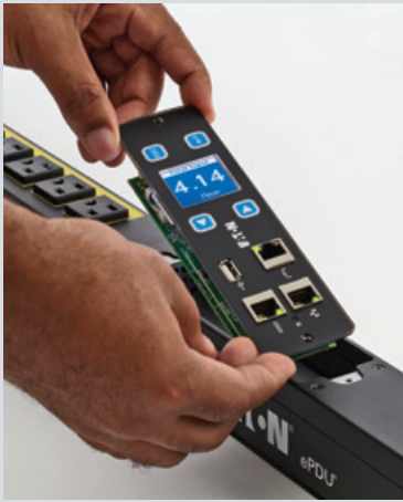
Module being removed without removing power to the PDU
