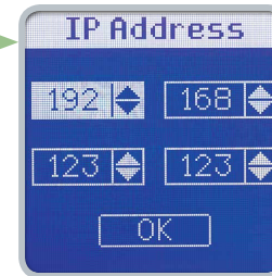
Manually set IP address without network connection
