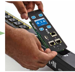
Module being removed without removing power to the ePDU
