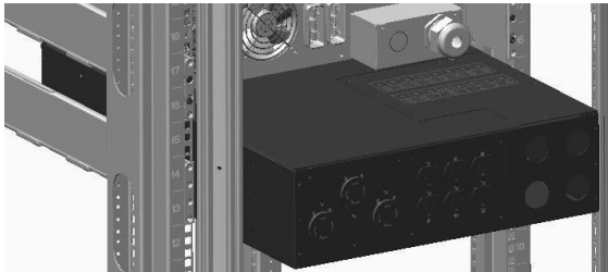
Figure 3. Push BPM into the Rack
