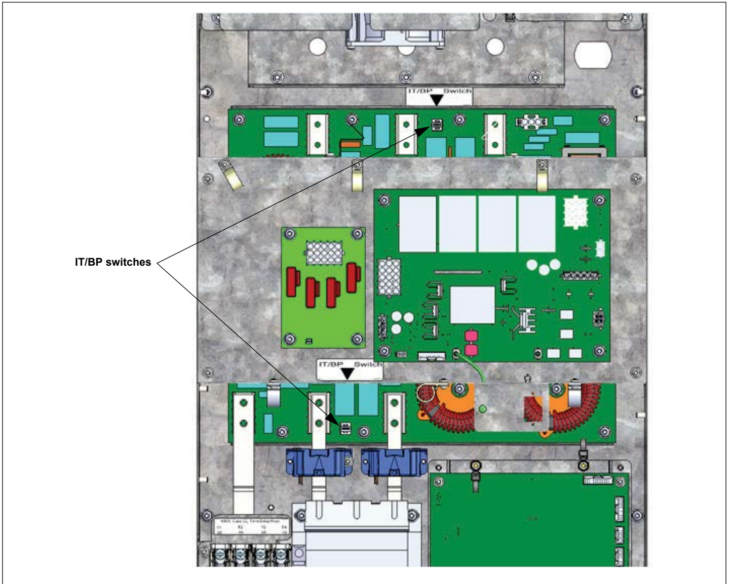
Figure 24. IT/BP switch locations on 60 A and 120 A units
