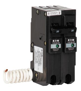
The BR surge breaker is designed to provide complete home surge protection for sensitive electronics and appliances from the damaging effects of surges. In addition to surge protection, the BR surge breaker is a functional 2-pole thermal magnetic breaker providing protection for overloads and short circuits.
