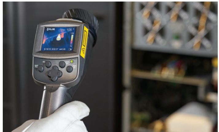
An infrared camera detects temperature variations—or hot spots—that can occur over time in electrical wiring and components.
