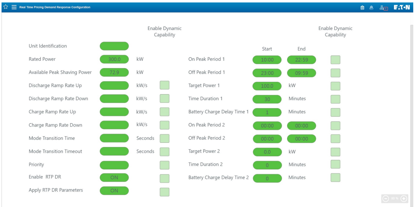
Figure 16. RTP DR Configuration Operational HMI Example
