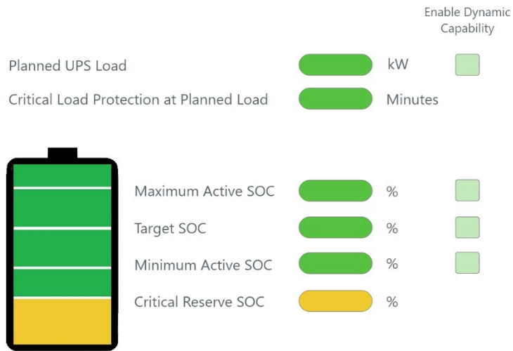
Figure 4. Battery SOC Configuration
