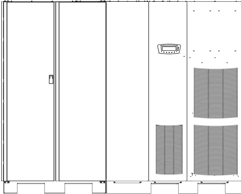
Figure 4-3. Line-up-and-Match MBM with a Eaton 9395 225-275 kVA UPS
