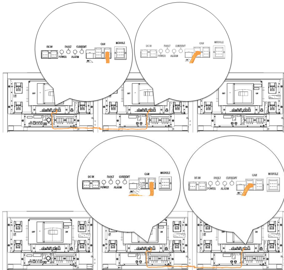
Figure 5-8: Signal Cabling Examples of Left Alignment of SMUs
