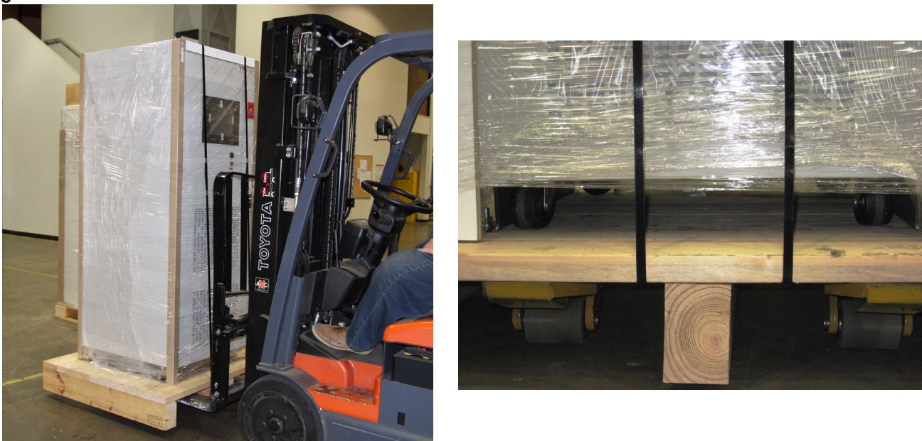
Figure 5 Removal of VDC with forklift
