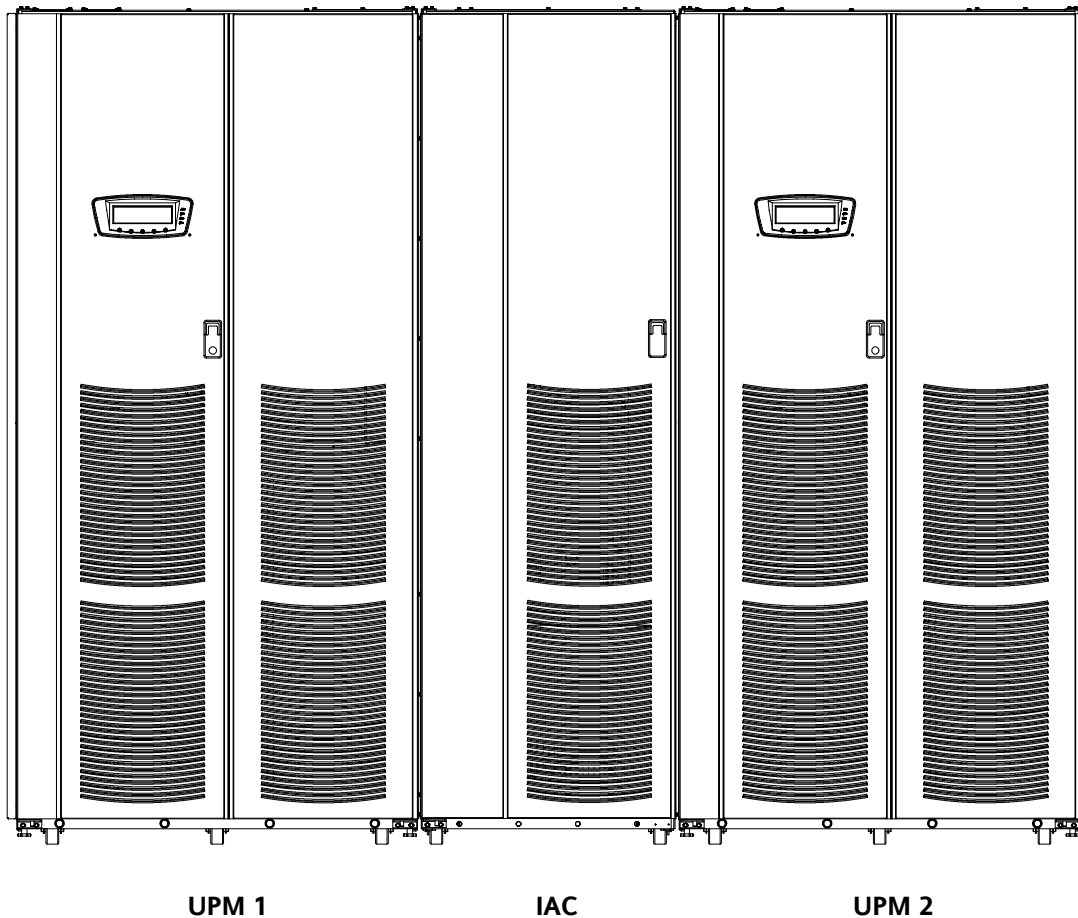
Figure 3-10. Two 100–160 kVA UPMs with Line-up-and-Match IAC
