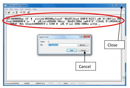
You will have to open the Windows task manager to "end task" 5PX Firmware Upgrade (07) – GUI version 1.21 And to allow the UPS to quit the bootloader mode, it is necessary to unplug it from Mains and to disconnect the battery cable.
