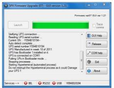
The UPS will first go under bootloader mode : the display is switched OFF
