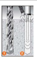
13. Insert Ramset C8 Resin into the holes using Ramset applicator Fill hole to 3/4 the hole depth ensuring no air pockets form
