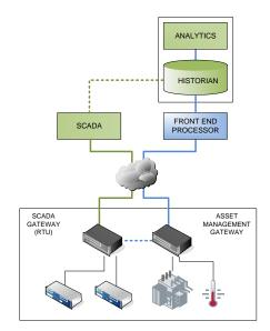
Figure 2: Parallel data path for non-operational data
