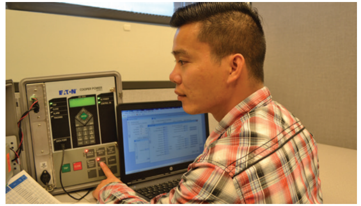
Distribution automation engineer reviews settings within capacitor control prior to field deployment using Eaton ProView NXG software™
