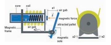
Figure 4. Role of air gaps in absorbing transient energy
