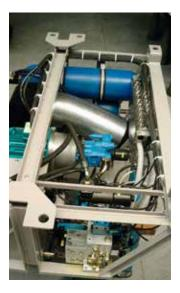
Eaton's Hydraulics Power Units contain PVM piston pumps, slip-in cartridge valves, servo valves and Eaton's filtration products HP.170 and HP.91
