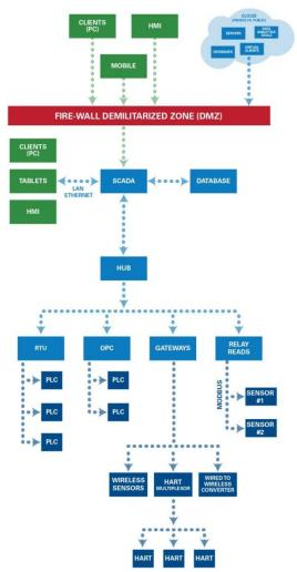
Fig. 6 - Traditional sensor network leveraging SCADA
