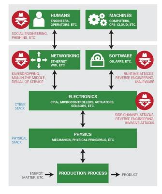
Fig. 5 – Typical cyber-physical production architecture and vulnerabilities
