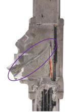
Fig. 12 Drain seal fitting showing the lack of any draining capability when the drain tube is covered with sealing compound.
