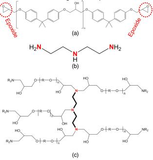
Fig. 5 Examples of reagents for an epoxy resin (a), hardener resin (b), and a cross-linked epoxy (c).
