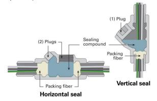
Fig. 4 Horizontal (left) and Vertical (right) seals showing the placement of the packing fiber.
