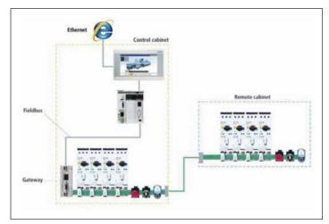
Figure 5. Device-level wiring systems use flat multiconductor cables to connect components, replacing bulky wiring ducts found in conventionally wired control panels
