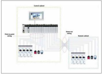
Figure 4. Device-level wiring systems use smart modules that connect standard motor control components via flat cable to a gateway module, which connects to a standard fieldbus on the PLC's CPU
