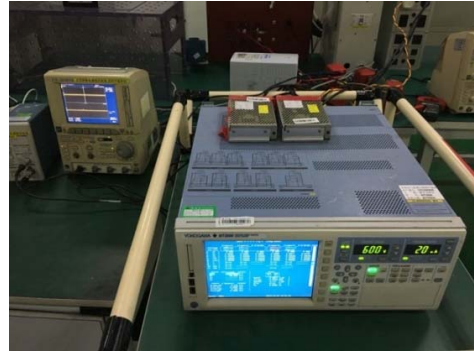
Figure 15: Experimental setup of 4.6kW ASD system with data acquisition using Yokogawa WT3000 precision power analyzer.
