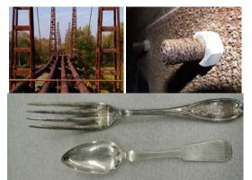
Fig. 1 Examples of common corrosion such as pipeline/bridge structures and bolts rusting [3] and silver tarnishing.
