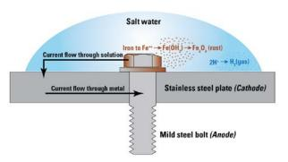
Fig. 4 Schematic description of a galvanic corrosion cell.
