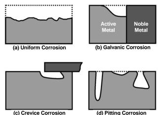
Fig. 2 Schematic representations of selected forms of corrosion, (a) uniform corrosion, (b) galvanic corrosion, (c) crevice corrosion, and (d) pitting corrosion
