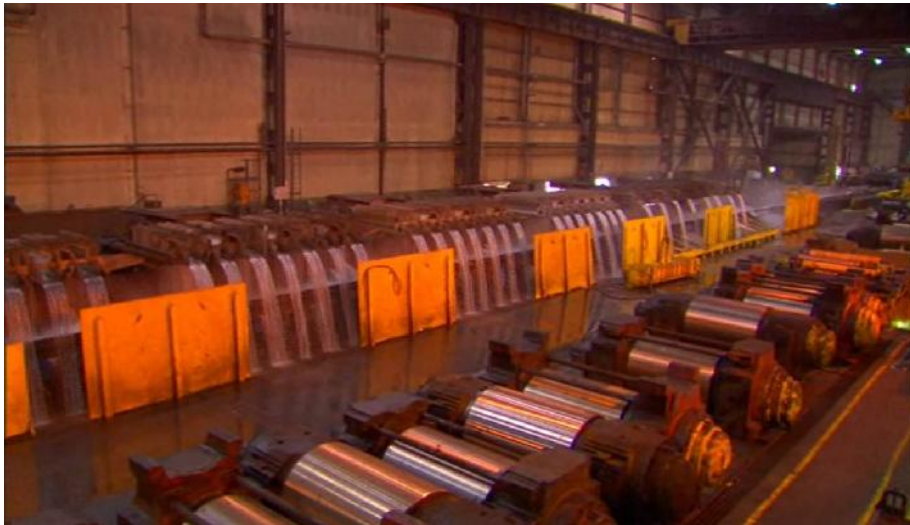
Fig. 1: Mill ROT system designed to cool hot strip to coiling temperatures between 1,000°F and 1,250°F.
