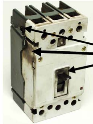
Fig. 4: Photo from IEEE Standard 1458 showing visible external damage to a breaker case, a stated reason to remove the breaker from service.
