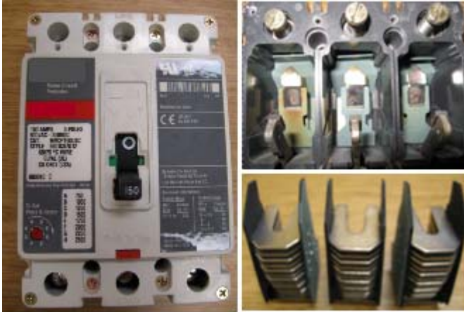
Fig. 12: Photos of Breaker 4919-1 clockwise from upper right; external breaker case, main moving and stationary contacts, arc-chute assemblies.
