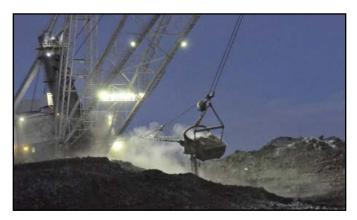
Fig. 5: Mine site dragline with 16 LED floodlights installed
