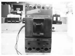
Figure 1. HKA Breaker Repaired by Third-Party Refurbisher, Following Testing
