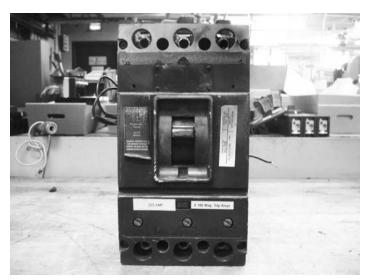
Figure 8. Third-Party Refurbished Breaker Failed to Interrupt on Short-Circuit Test
