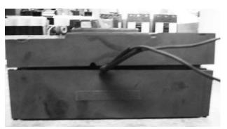
Figure 2. Breaker Cover Separated from Base During High Fault Test
