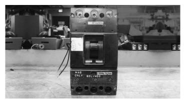
Figure 14. HKAM Mining Breaker Modified by Third-Party Refurbisher
