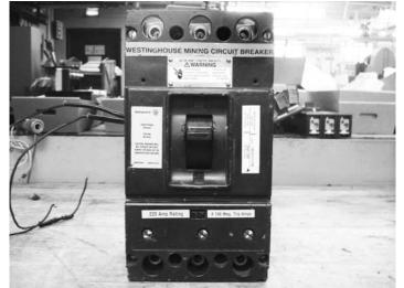
Figure 10. Third-Party Refurbished Breaker After Failing Load Endurance Test
