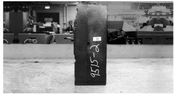
Figure 15. Undervoltage Release Accessory Malfunctioned; Breaker Could Not be Reclosed
