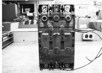
Figure 7. Breaker After High Fault Test; Conductor Material Overheated and Melted Away
