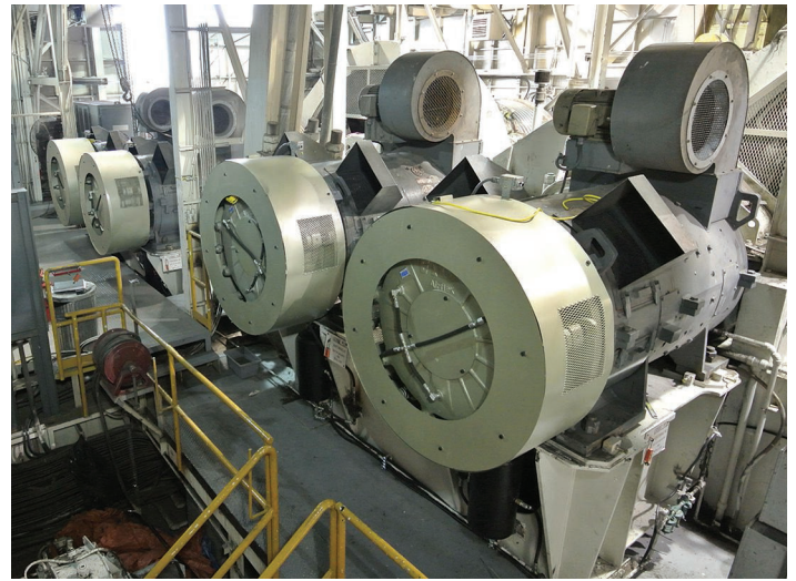
Eaton's Airflex 138 Floating Housing Brakes installed on mines dragline excavator.
