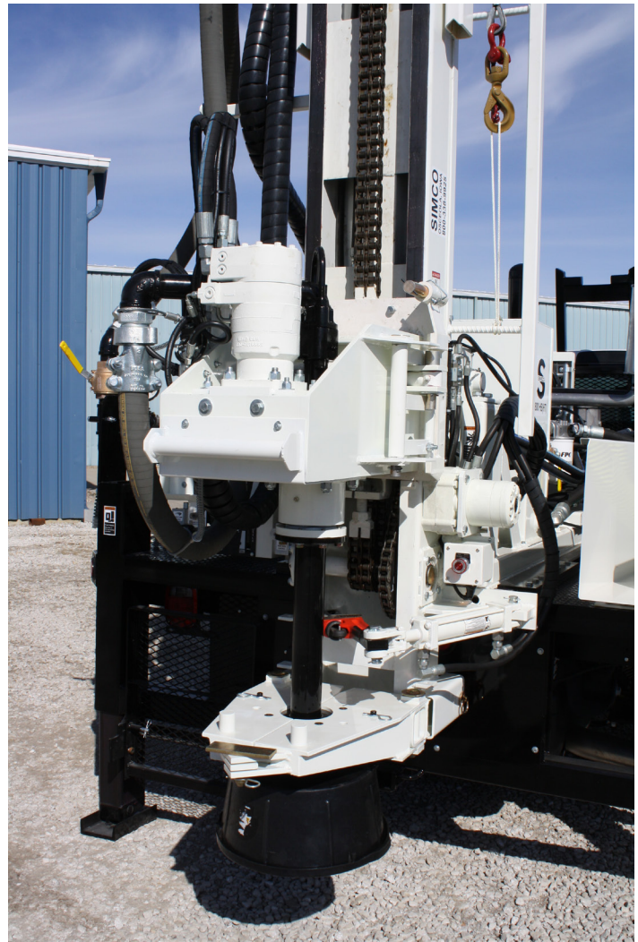
Eaton's Char-Lynn HP30 high-pressure motor powers the standard drillhead on SIMCO's 2800 HS (HT) drilling rig.
