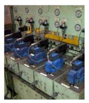
Eaton's Vickers KBHDG5V-7 Series two-stage, servo-proportional directional valves provide accurate high speed profiling on valve stands.
