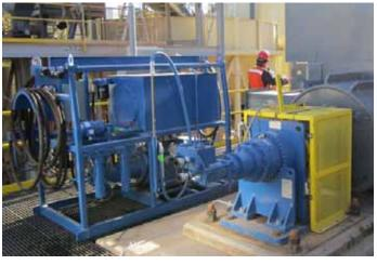
Eaton's new hydraulic inching drive includes a 75-hosepower hydraulic power unit skid and an Eaton Char-Lynn 6000 Series hydraulic drive motor.
