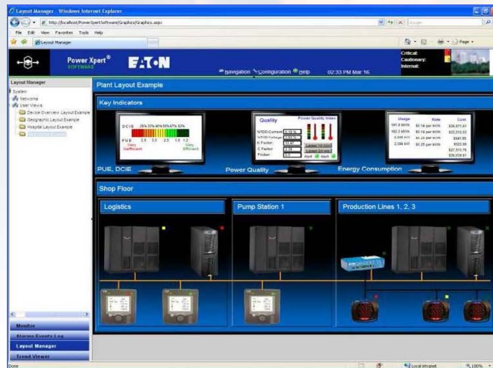
Figure 2: Power management software enables data center personnel to perform many tasks remotely rather than expose themselves to arc flash dangers.
