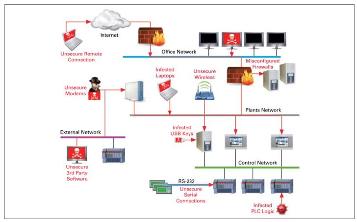
Figure 2. Paths to the Control Network from a Corporate IT Manager's Perspective
