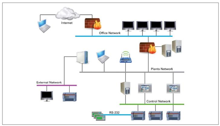
Figure 1. Paths to the Control Network from an Engineer's Perspective
