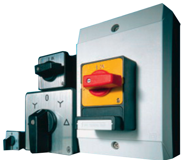
Figure 34: T rotary cam switches, and P1 and P3 switch-disconnectors are certified as industrial control equipment per UL 508 and CSA-C22.2 No. 14-05 and additionally evaluated as motor disconnects. They can be used as individually enclosed isolating disconnect switches local to the motor when installed on the load side of the motor branch circuit protective fuse. A line side motor disconnect switch must be certified per energy distribution standards such as UL 489 and CSA-C22.2 No. 5-09.
