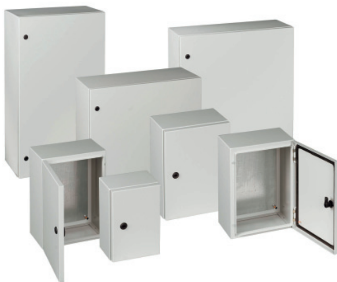
Figure 38: The CS enclosure series is a line of wall mounted steel enclosures certified for the US and Canadian marketplace. Up to 44 different enclosure sizes are available, ranging from 250 x 200 x 150 mm to 1200 x 1000 x 300 mm. The enclosures are UL/CSA Type 1 and 12 rated, for industrial indoor usage.
