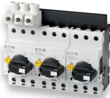
Figure 19: The manual motor controller on the left, with the incoming terminal block, is fully certified as a “Manual Self-Protected Combination Motor Controller”, also commonly referred to as a “UL 508 Type E Starter”. This additional terminal block on the incoming supply side of the controller provides the larger electrical clearances required for this application. The single terminal is allowed to feed additional self-protected controllers in this manner, as long as they are inter-connected using busbar accessories specifically listed for this purpose. This particular configuration provides both a useful way of complying with North American requirements and a space saving feature typical of similar designs conforming to IEC/EN standards. This solution is applicable in solidly grounded power distribution networks. Applications in Canada would require each open panel mounted self-protected controller applied in this manner to be equipped with a padlockable knob. These controllers are suitable for installation in motor branch circuits only.
