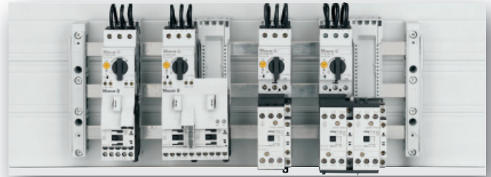
Figure 39: SASY 60i is a modular busbar system designed for optimum distribution of electrical energy in industrial control panels - safe, and space saving -. The use of busbar adapters and component shoes allow for quick and efficient mounting of incoming and outgoing power components as well as many varieties of motor starters. The photo shows an array of mounted and wired components (IEC/EN).
