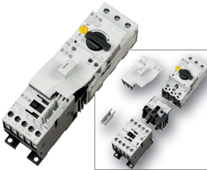
Figure 13: Efficiently combining motor starter components using plug-in mechanical and electrical connector kits. This type of construction is certified, just like the traditional way of combining components using hard wire. This type of motor starter requires an additional back-up protective switch per North American standards, or it can be applied as a stand alone Type E or F combination controller when equipped with a large spacing BK25/3-PKZ0-E supply terminal. (Refer to Figure 19).
