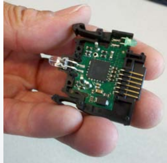
Onboard communications inside each Eaton SmartWire-DT module helps improve speed to start-up over traditional control panel wiring. Courtesy: CFE Media
