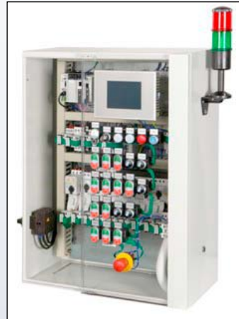
SmartWire-DT is a control panel wiring solution that allows OEMs to simply connect motor control devices on a panel using a flexible flat cable, eliminate traditional point-to-point control wiring, help protect control interlocking, and provide data monitoring of connected motor loads.
