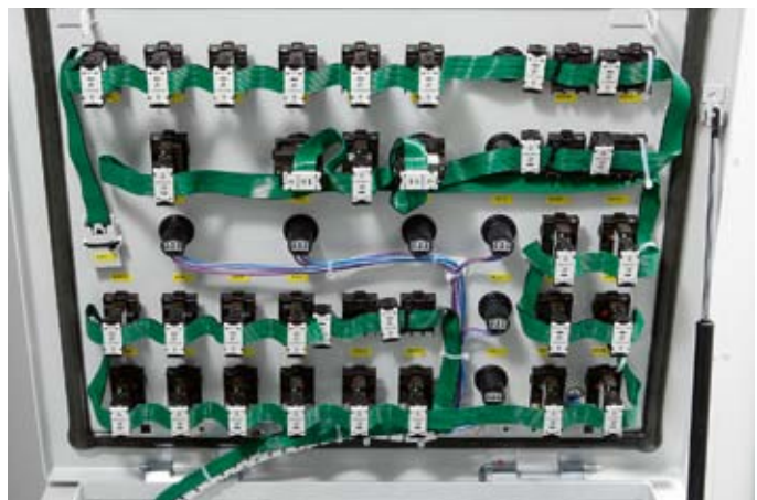
The Power of One: A complete system is being developed jointly by Eaton Hydraulics and Eaton Electrical, enabling both hydraulic and electrical components to be connected to SmartWire-DT and monitored centrally
