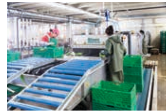
The system for the Pfälzer Renner vegetable production plant is capable of cleaning and cutting different vegetables, depending on the degree of soiling
