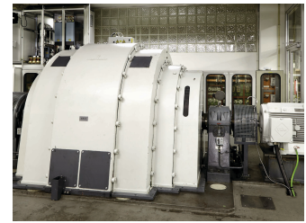
The surge generator in the test laboratory of I 2 PS GmbH, right, the new asynchronous motor, left behind the open switching cabinet with the Eaton drive solution.
