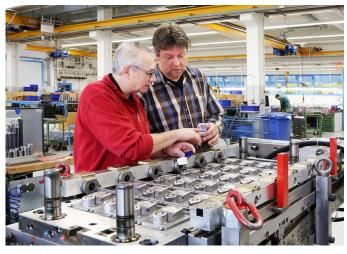
At its German headquarters, WPPG produces its own tools for its injection molding machines.
