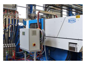
The switch cabinet also contains Eaton's XI/ON modular I/O system which handles the data exchange with the locking system of the guard door, the position sensors or between the tool and the injection molding machine.
